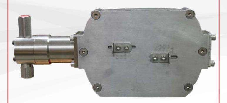
Sidewinder Pumps introduces our new Stroke Length Adjuster for AC / Solar Pump lines. The progressive design allows for 0-100% adjustment while pump is running. This provides accurate flow control options especially on duplex pumps with different size plungers. Setting the Stroke Adjuster to 0 will allow maintenance to be done to that pump without having to take pump out of service. The Stroke Adjuster can be retrofitted to existing pumps.
