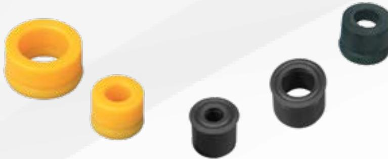
**Sidewinder AC pumps use the same seal arrangements as our pneumatic pumps. Chevron or adjustable style packing allows the operator to over tighten the packing creating excessive drag on the plunger, resulting in greater energy draw, which shortens battery life. With our unique design, seals can be changed in matter of minutes without having to dig them out with tools that can mar or damage the seal gland.**
