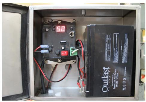
Electronic Timer with digital read out, provides ease of setting pump flow and has port for optional temperature probe
