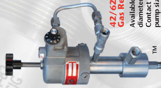
42/62/82 E Series Pump Micrometer Stroke Adjuster feature with graduated scales for precise flow control. Flows to 275 QPD Pressure to 10,000 PSI Available in 1/4", 3/8", & 1/2" diameter plungers
